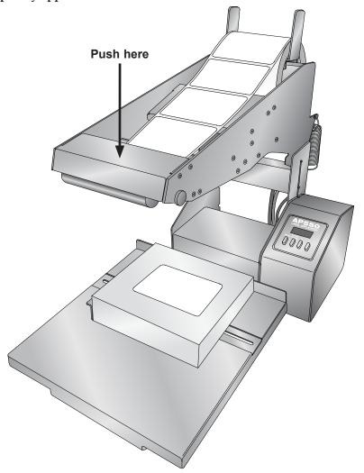
**Note:** If you stop or delay when bringing the arm toward the container, the label could be ejected before the arm reaches the container. Excessive force may cause the platform to stall.
