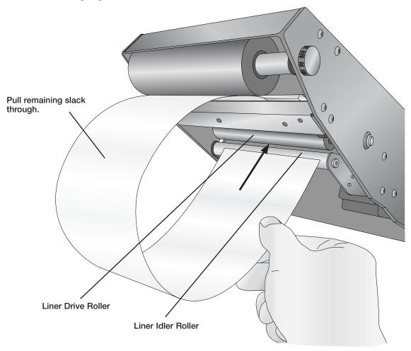
12. Feed the leading edge of the label stock under the stock coming off the roll. Align the leading edge of the label stock so that it is directly under the stock coming off the roll. Pull it tight.
